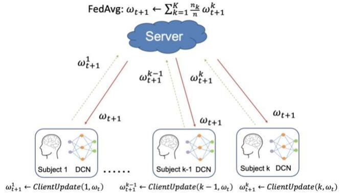
Figure 1: The Architecture of Fed-DCN
